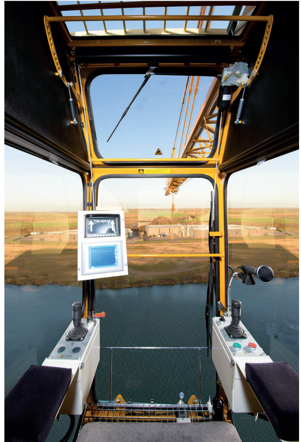
Crane Cabin equipped with trolley camera display and touch screen.
